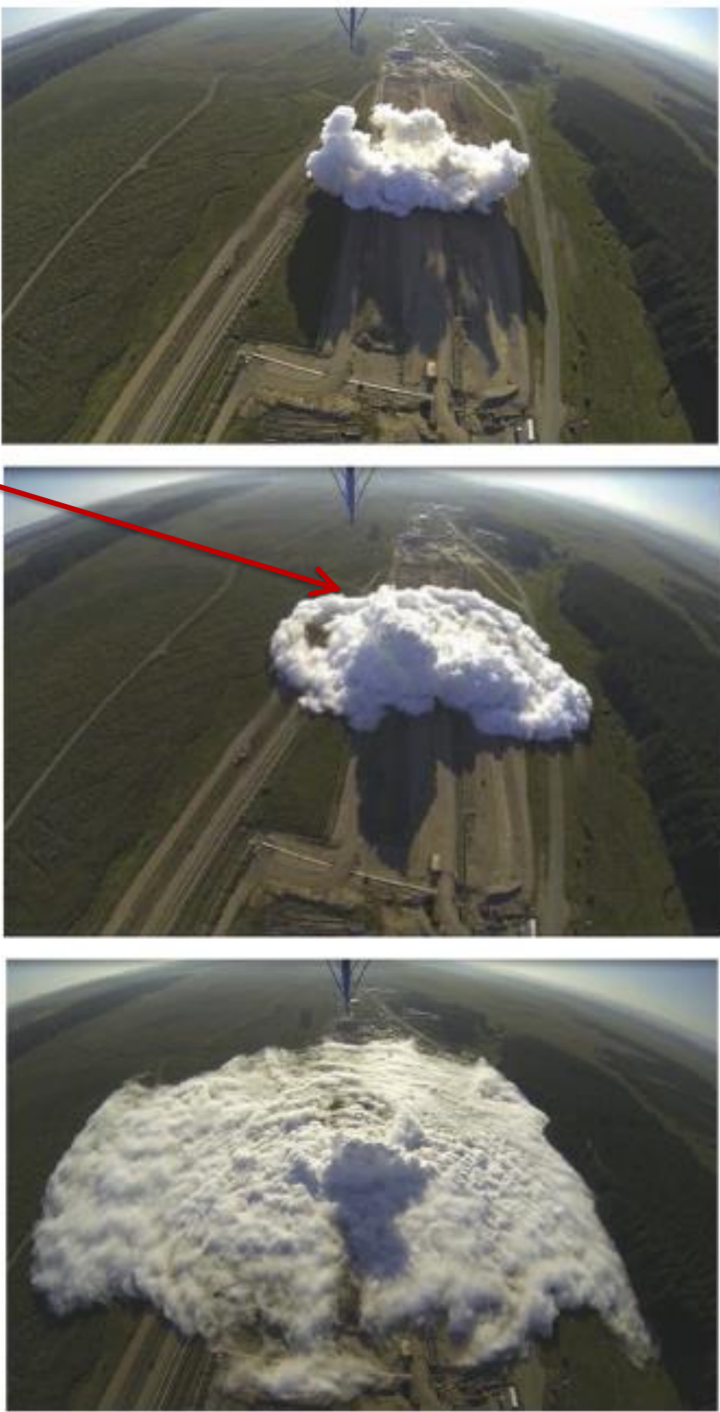
Fig. 4. The visible cloud at 10 s (top), 30 s and 120 s (bottom) after the rupture.
